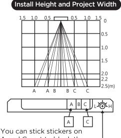
A and C part to block the infrared ray.
